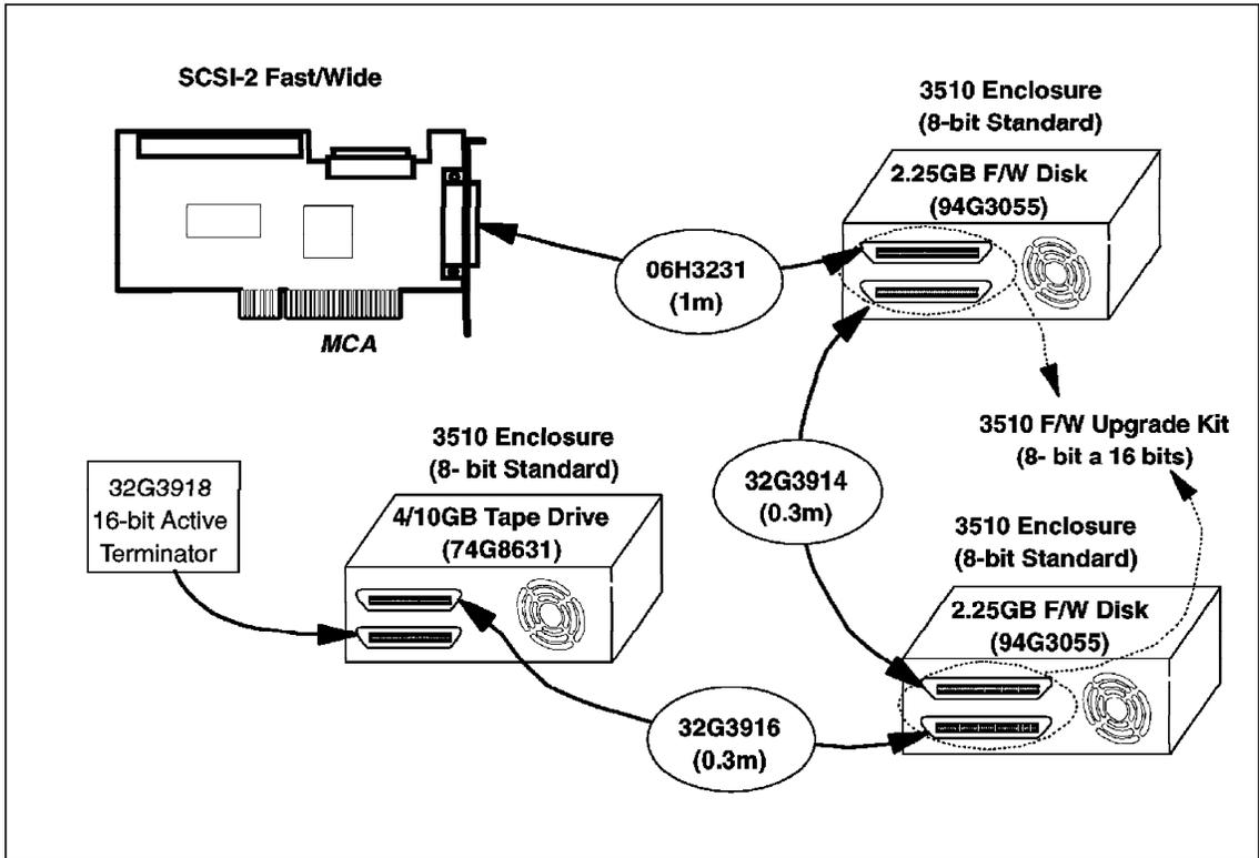
Figure 40. External 16 and 8-Bit SCSI Configuration
