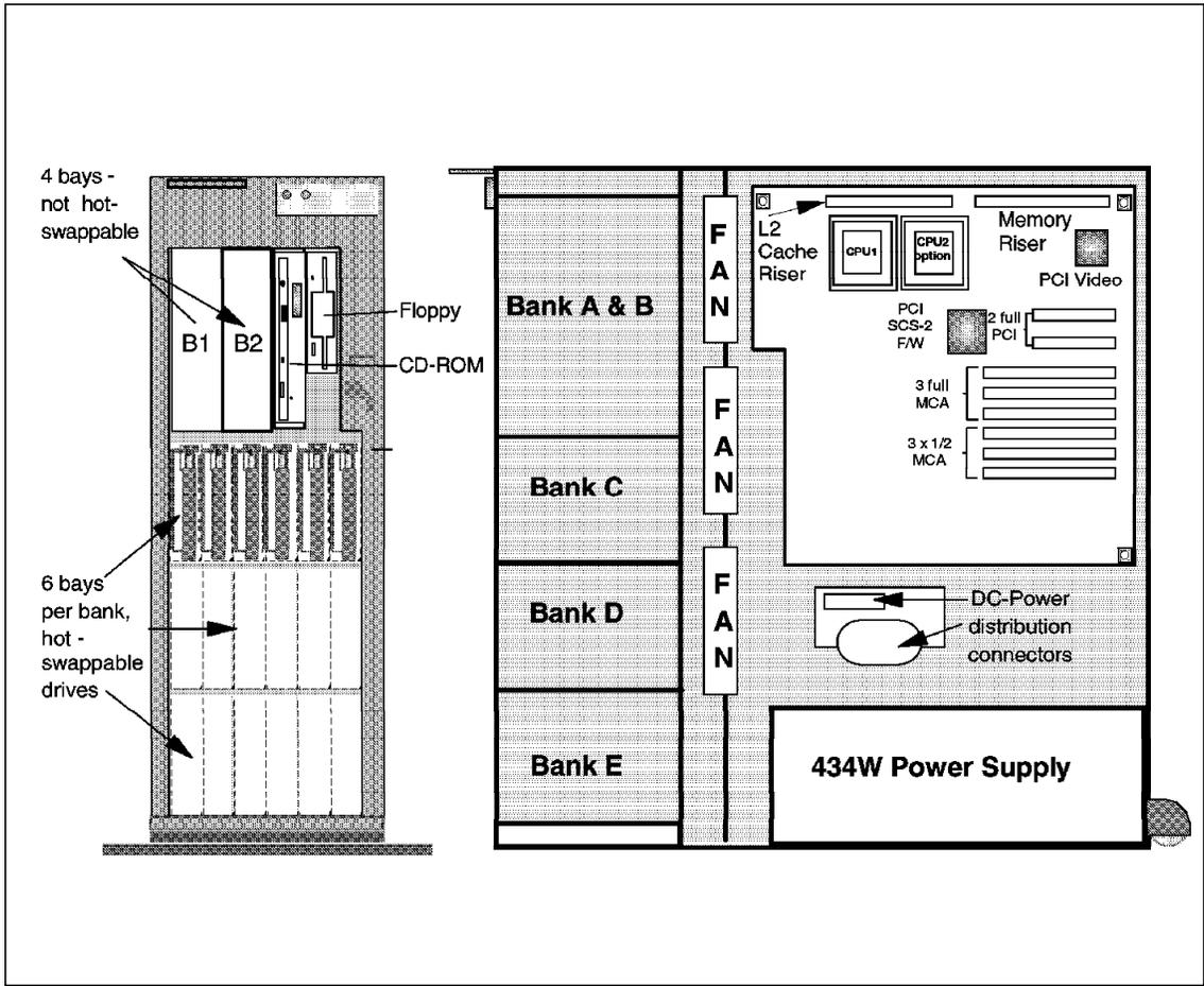
Figure 29. IBM PC Server 520 MCA/PCI - Mechanical Design
