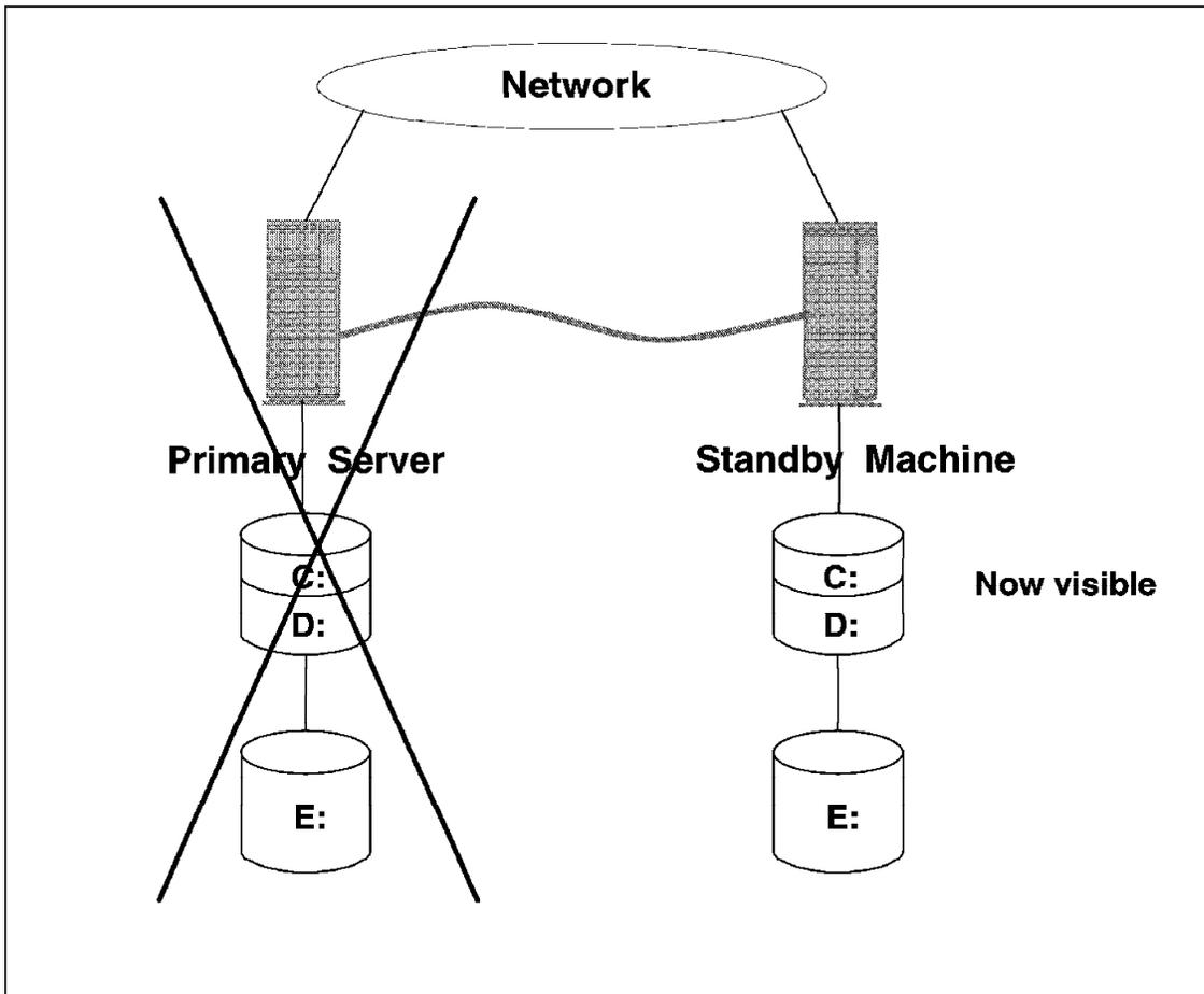
Figure 67. Switch Over to the Standby Machine
