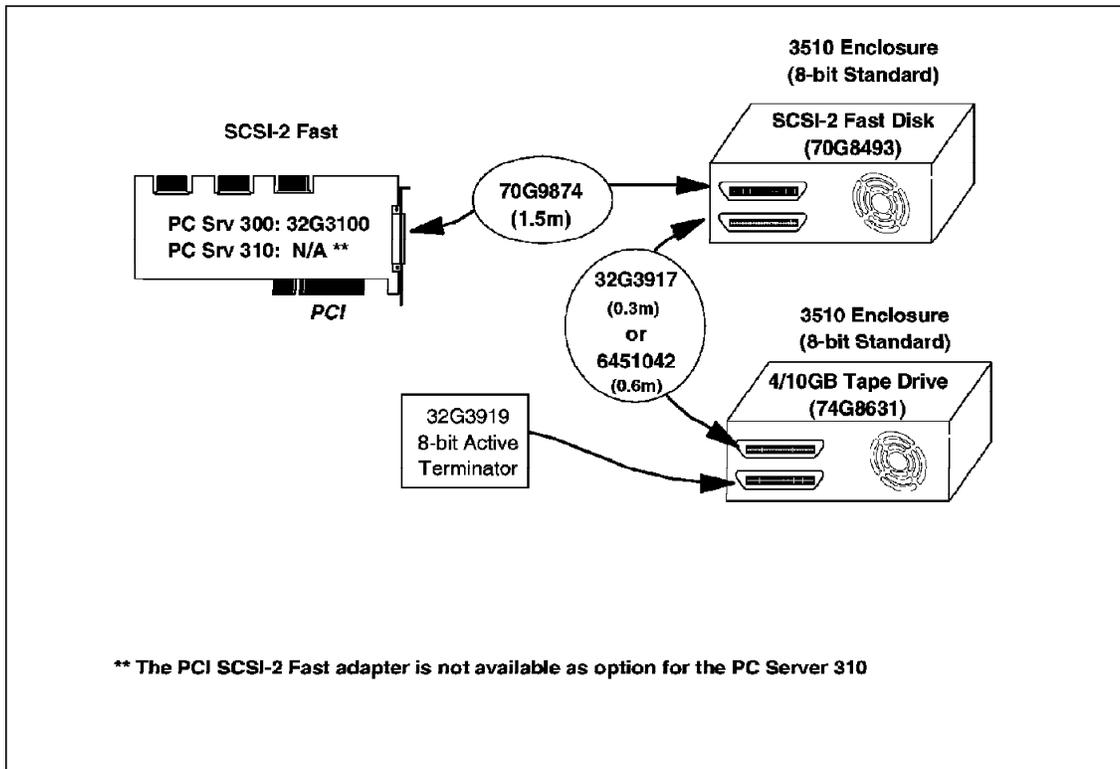
Figure 37. PC Server 300 External Cabling Example (PCI SCSI-2 Fast)
