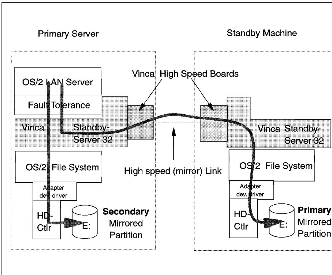
Figure 64. StandbyServer 32 for LAN Server Concept
