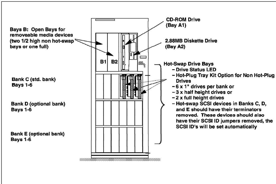
Figure 22. PC Server 500, 520, and 720 Internal Bay Structure
