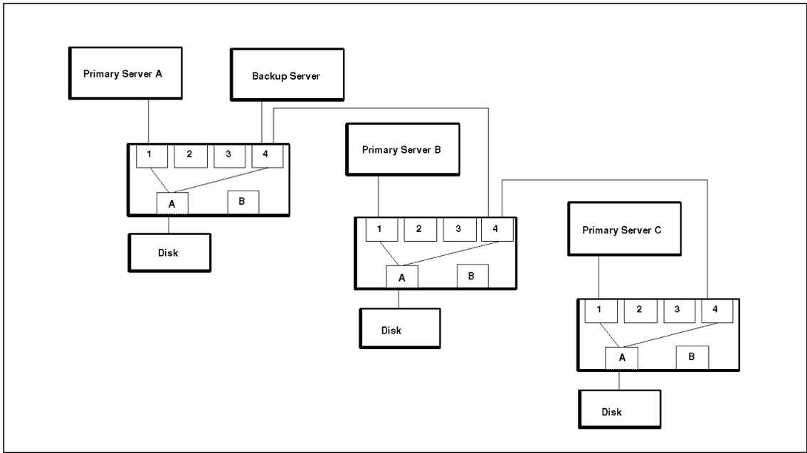
Figure 71. APPLIED Concepts (Backing up Multiple Servers)
