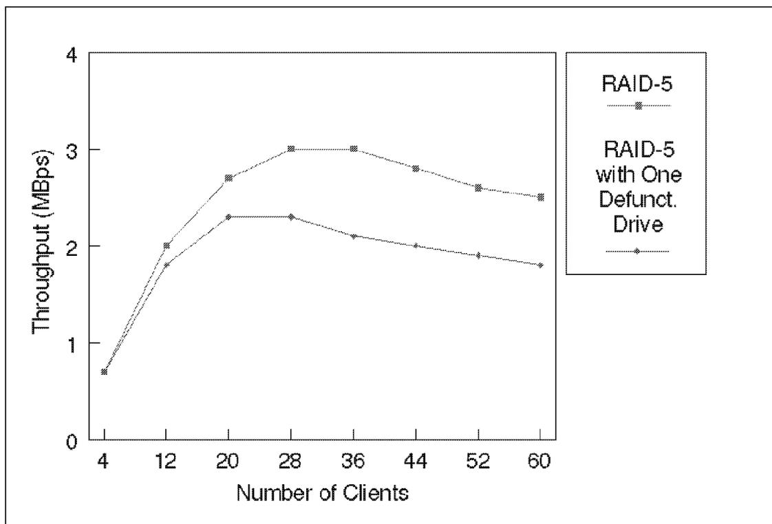
Figure 61. IBM PC Server 320, RAID-5 with One Defunctional Drive
