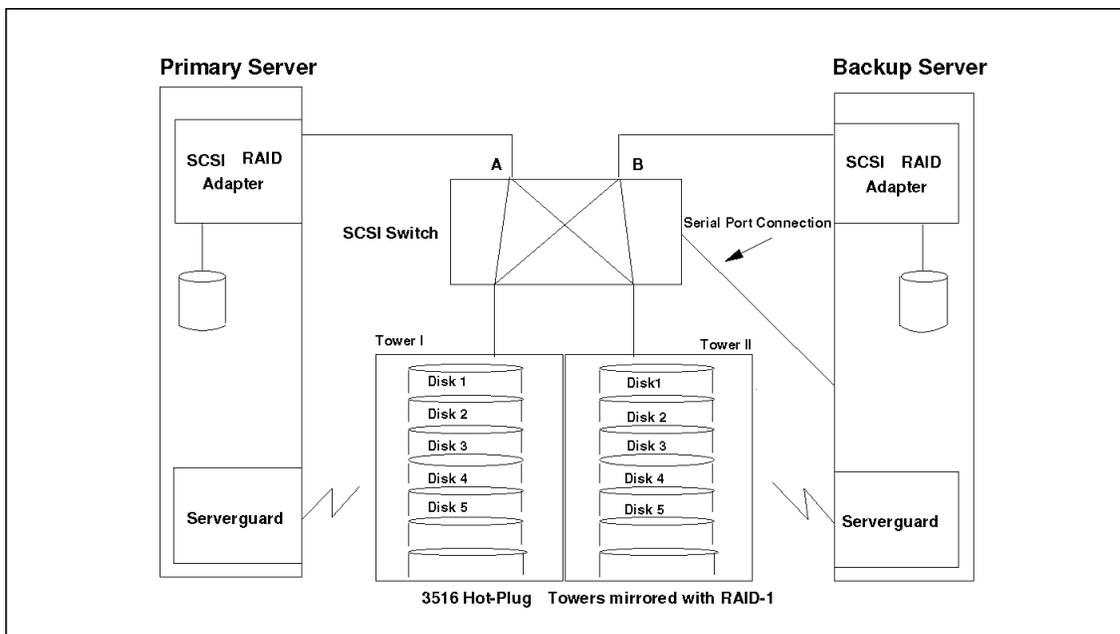
Figure 74. High Availability Server (External Mirrored RAID-1 Towers)
