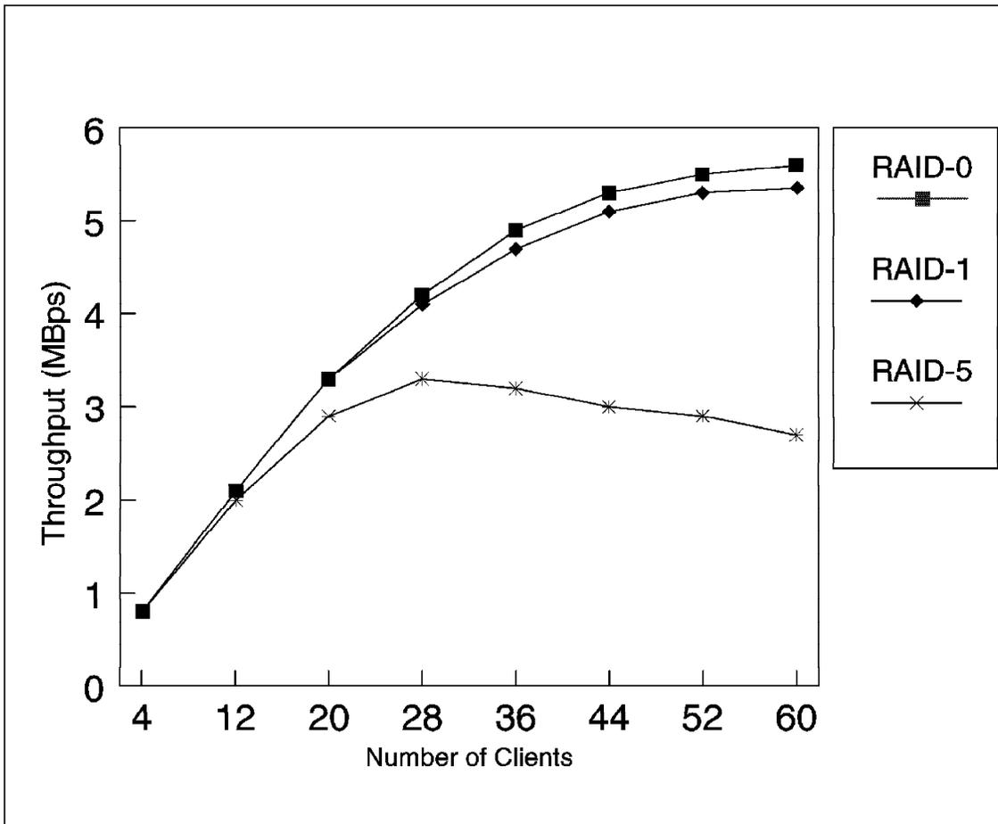
Figure 54. IBM PC Server 500, RAID-0, 1 and 5 Throughput
