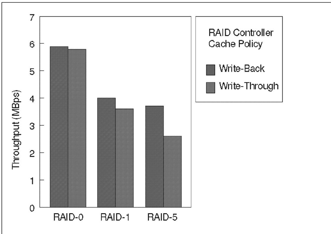
Figure 60. IBM PC Server 320, Write-Back versus Write-Through
