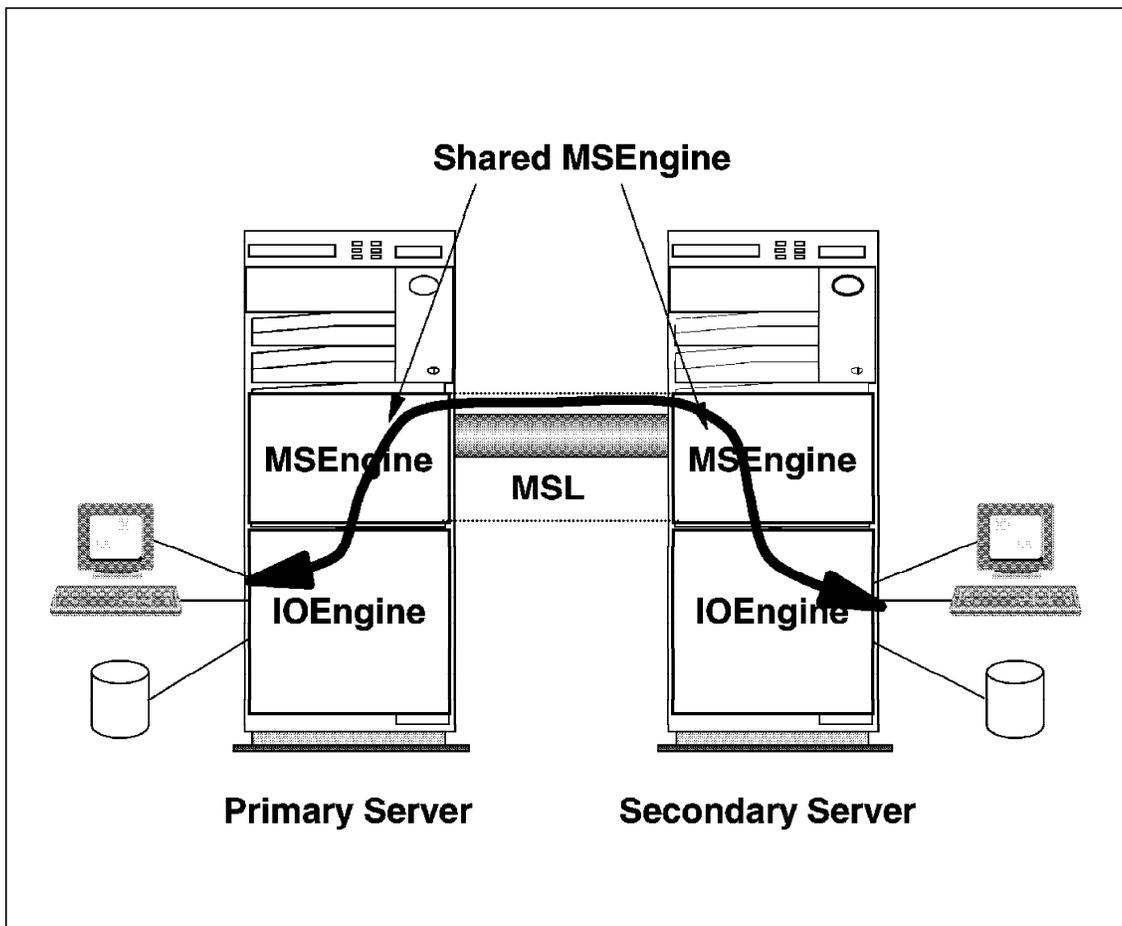
Figure 63. SFT III IO- and MEngines
