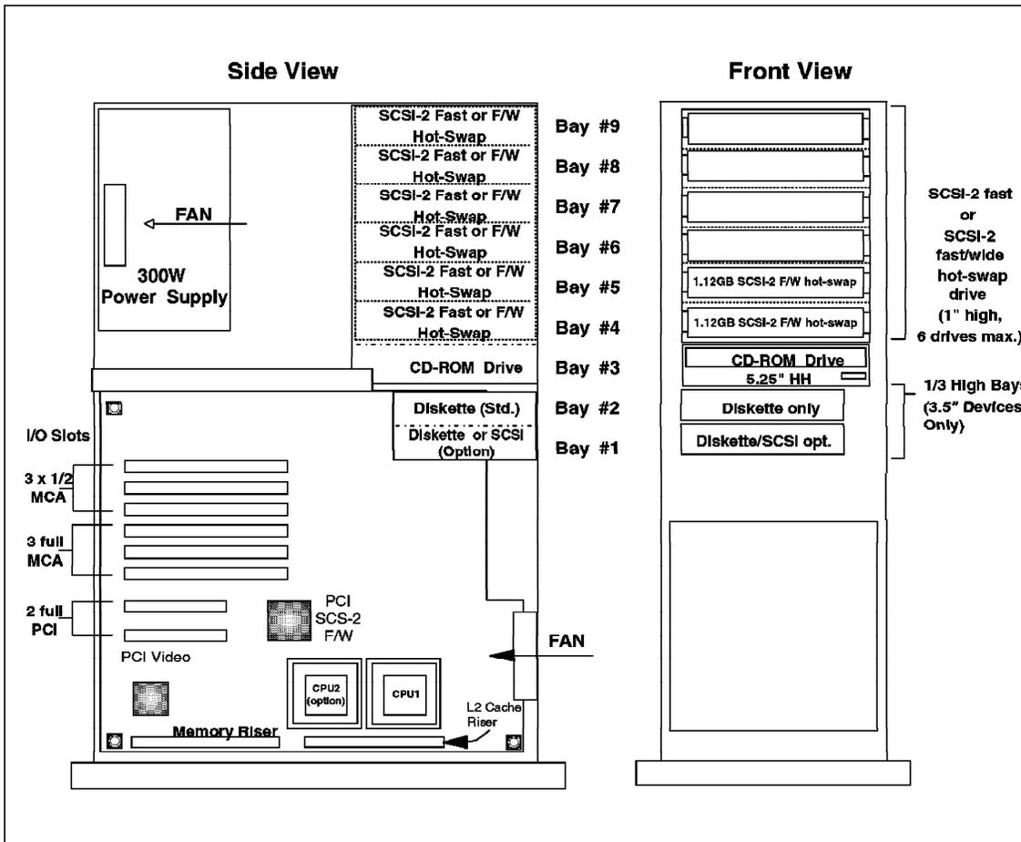
Figure 20. IBM PC Server 320 Array Mechanical Design
