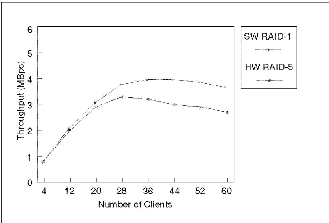
Figure 53. Performance Software RAID-1 versus Hardware RAID-5
