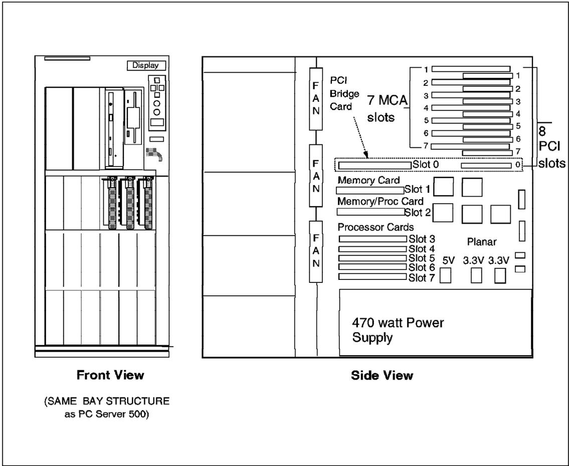
Figure 23. PC Server 720 and 720 Array Mechanical Design
