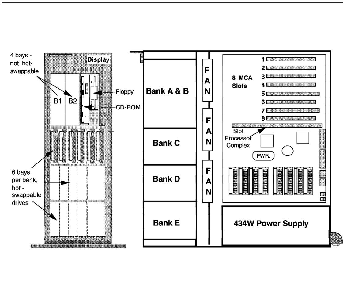
Figure 24. IBM PC Server 500 - Mechanical Design
