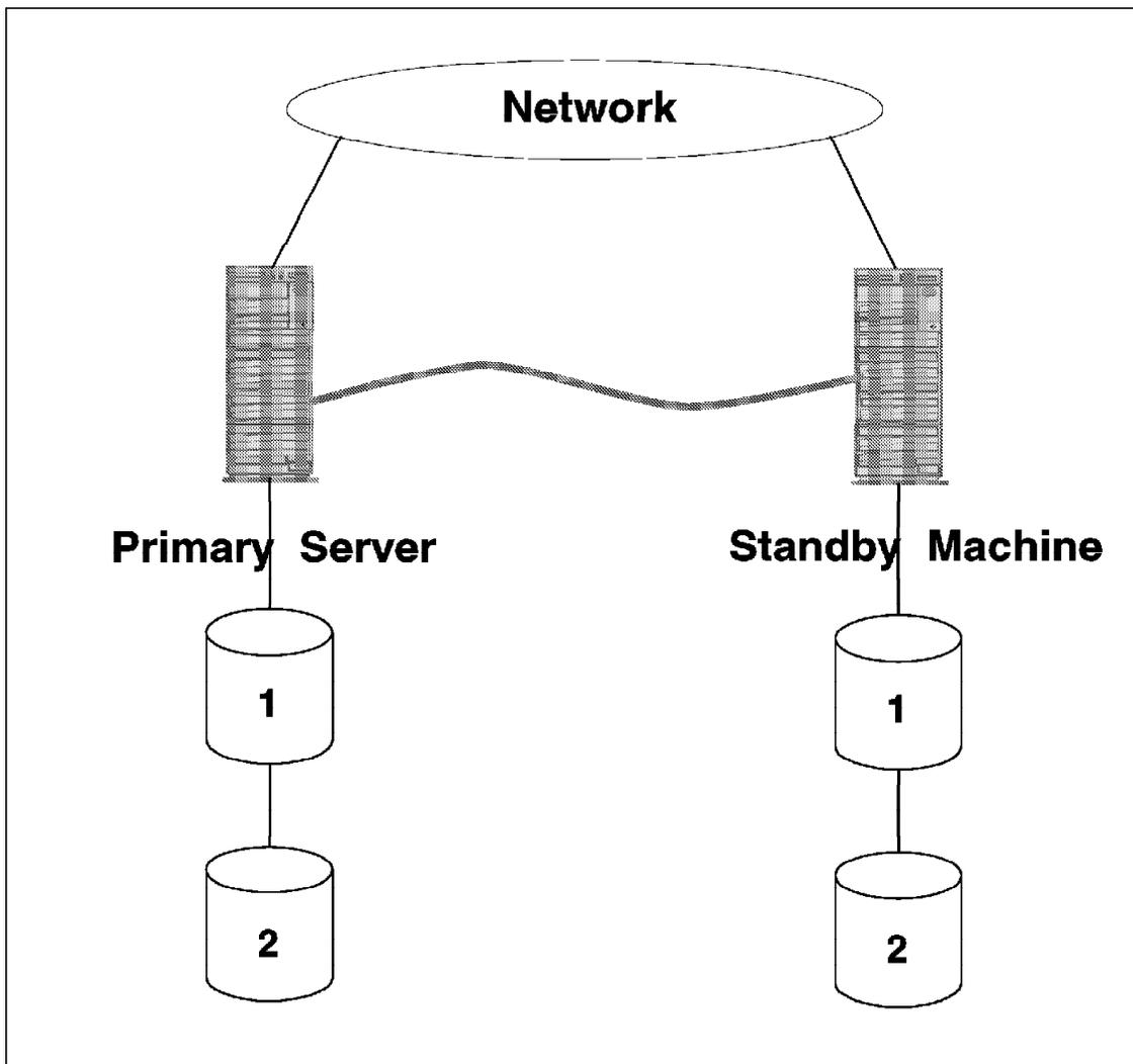
Figure 65. StandbyServer 32 for LAN Server Minimum Configuration
