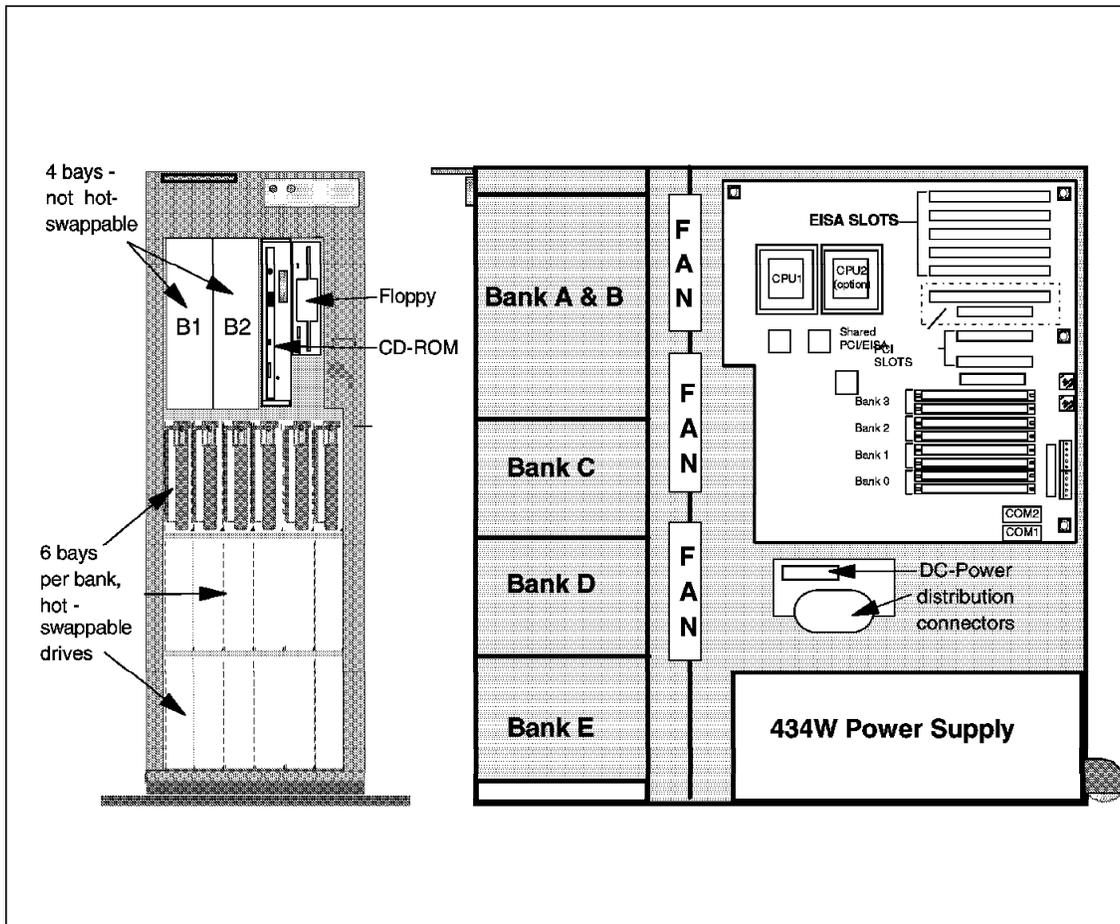
Figure 27. IBM PC Server 520 EISA/PCI - Mechanical Design
